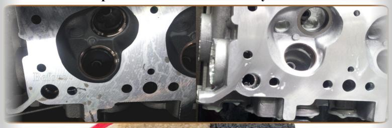
Slots, Edge & Crosshole DeBurred photos of Aluminum Components
